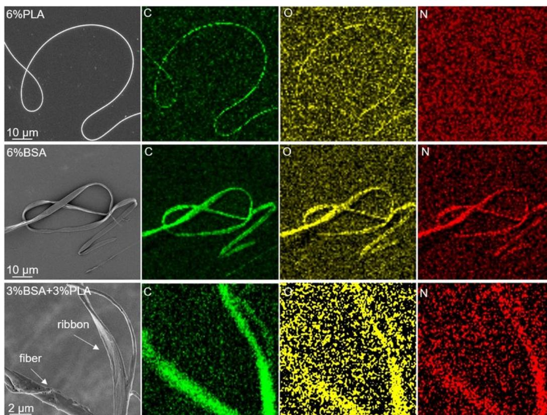
*Fig.1 : EDX analysis of the fibers made of PLA (top row), BSA (middle), and the PLA-BSA blend in equal proportions (bottom). The color mapping corresponds to the chemical elements, with the carbon, oxygen, and nitrogen shown in green, yellow, and red*
